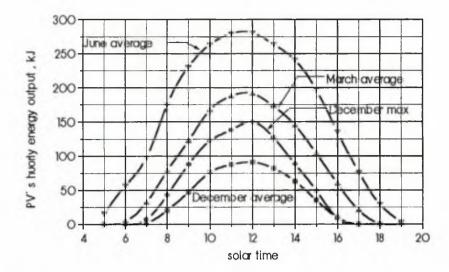
Figure 3. PV panels hourly energy output, in kJ, supplied to the batteries, for the duration of the average December day, the max December day, the average March day and the average June day
