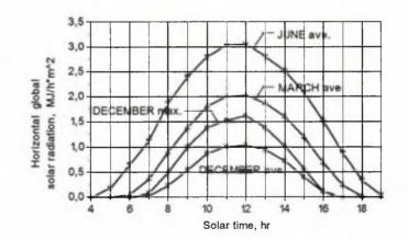
Figure 2. Global solar radiation hourly distribution on the horizontal plane for the average December day, maximum December day, average March day, and average June day in Athens, from measurements at the T.E.I. station
