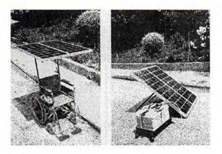
Figure 6. A front view with the PV panels on their mountings and the speed-direction switch controller on the right arm rest
