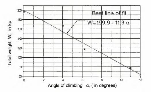
Figure 1. Wheel chair's climbing ability, measurements and best line of fit
