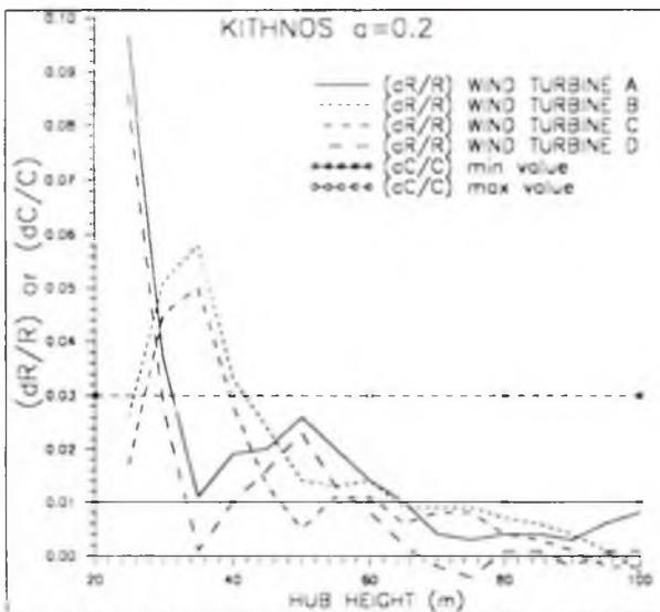
**Fig.8: WT's relative cost and revenue changes with hub height.**
