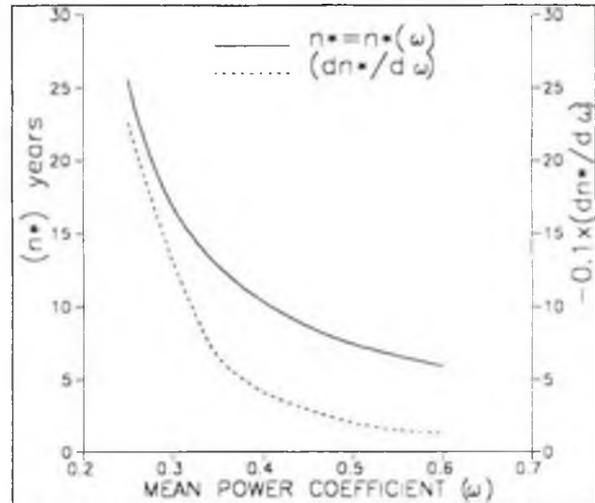
Fig.7: Influence of "ω" on the pay-back period of a WT installation.
