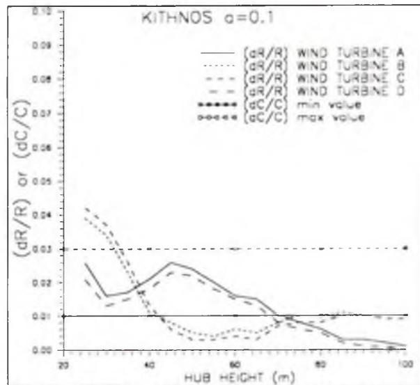
**Fig.9: WT's relative cost and revenue changes with hub height.**
