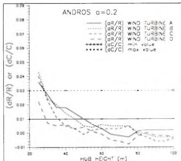
**Fig.10: WT's relative cost and revenue changes with hub height.**
