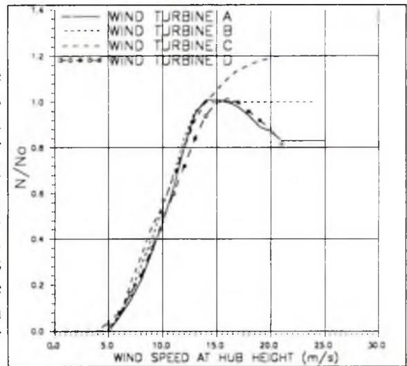
Fig.1: Wind Turbine Power Curves
