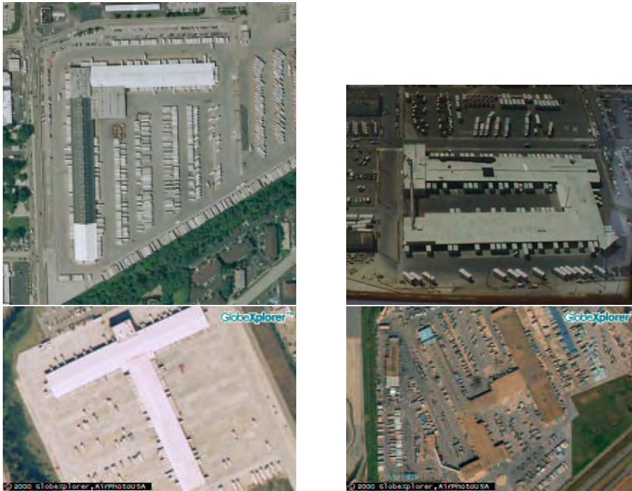
Figure 13.4: Crossdocks have been built in a variety of shapes. Clockwise from upper left: An L-shaped terminal of Yellow Transport; a U-shaped terminal of Consolidated Freightways; a T-shaped terminal of American Freightways; an H-shaped terminal of Central Freight
