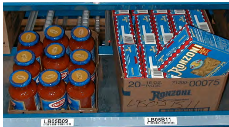
Figure 9.6: Pasta and tomato sauce are two skus that have “affinity”: Any customer ordering pasta is likely to order tomato sauce. Storing them together may reduce the work to pick the order.
